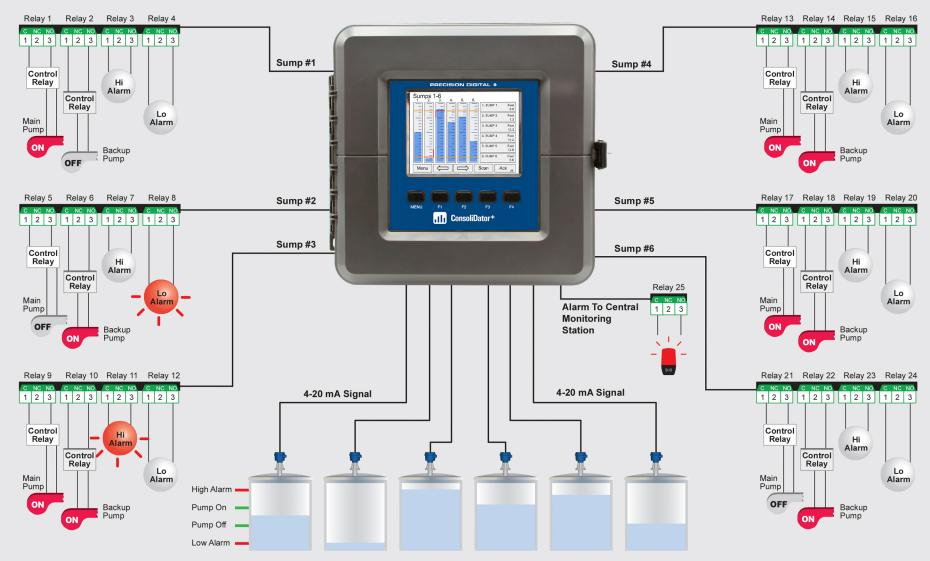
One ConsoliDator+ monitors and controls 6 sumps. All 4-20 mA inputs from the level transmitters are isolated and powered by the ConsoliDator+. Twenty four 10 A Form C relays control and alternate 2 pumps in each sump while providing high and low level alarms for each sump. One relay sends a signal to a central monitoring station when any sump goes into high alarm. Ethernet Modbus TCP/IP is available.
