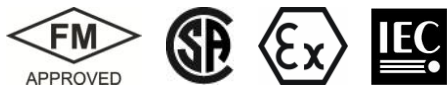
FM, CSA, ATEX, and IEC Marks Found on Some Hazardous Area Equipment
