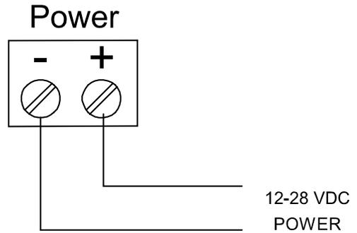
Figure 2. Power Connections
