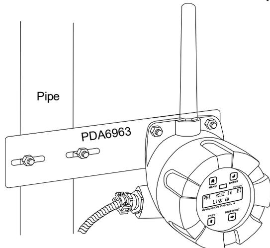
**Figure 11. PDA6963 Stainless Steel Pipe Mounting Kit**
