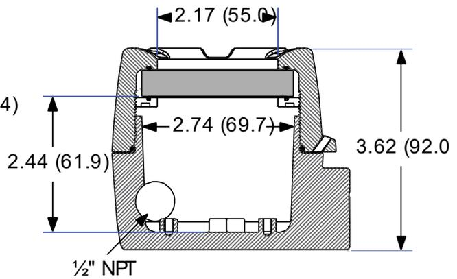
**Figure 10. Enclosure Dimensions – Side Cross Section View**
