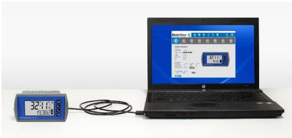
The easiest and quickest way to program your loop-powered feet & inches level meters is with the free, PC-based, MeterView XL software. The level meter connects to the PC with a USB cable that also provides the power to the level meter during programming. Programming files can be saved for later use.
