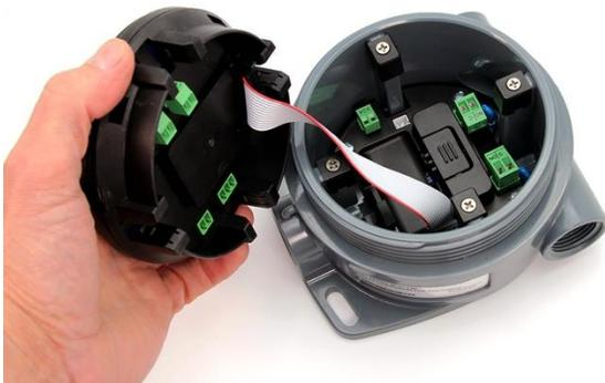
Options Module Mounted on the Bottom of Enclosure
