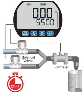
If set to automatic, then a delay before the next batch starts must be programmed.
