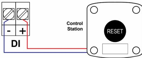
Figure 30. PDA2361-R Control Station Connected to PD6938
