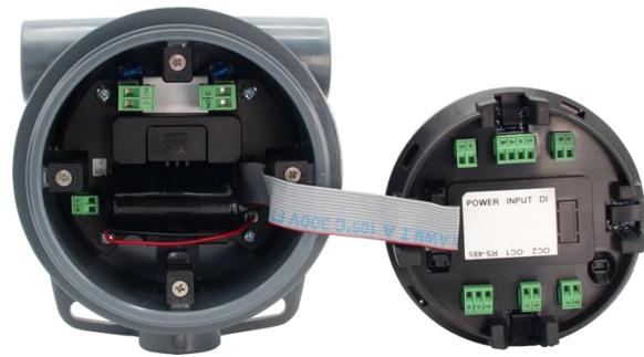
Options Module (Left) and Display Module (Right)
