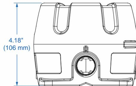
Figure 3. Enclosure Dimensions – Bottom View
