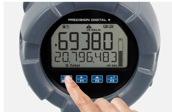
CapTouch buttons have two modes of operation: Normal and Delayed. Delayed mode prevents accidental trigger of the buttons. In the Delayed mode, the buttons enter into a low sensitivity state (sleep) and they ignore quick button presses after 20 seconds of inactivity. To wake up the buttons, press and hold any button for more than 2 seconds, the buttons respond normally.
