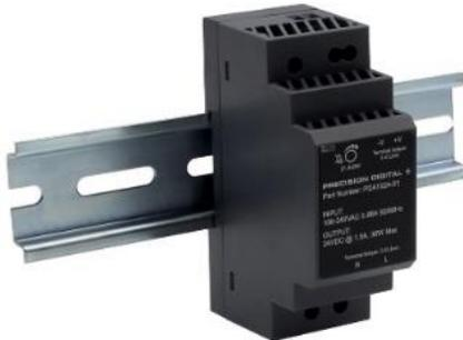
The PDA1024-01 is a DIN rail mounted 1.5 A, 24 VDC power supply that can be used to power the PD6938 and the 4-20 mA output.
