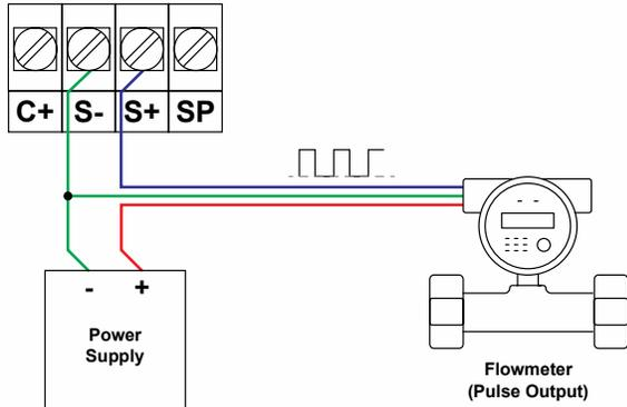
Figure 16. Flowmeter Powered by External Supply (Active)
