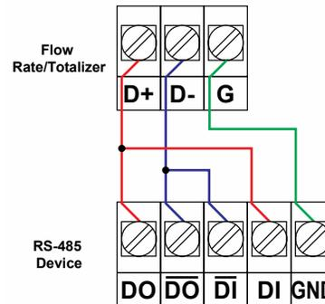
Figure 26. RS-485 4-Wire & Ground Serial Connections
