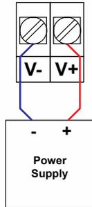
Figure 23. DC Power Connections
