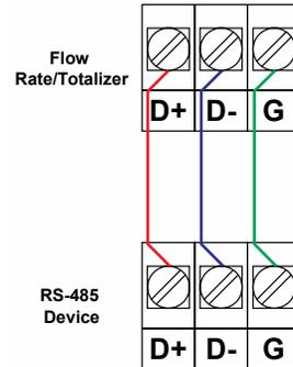
Figure 25. RS-485 2-Wire & Ground Serial Connections
