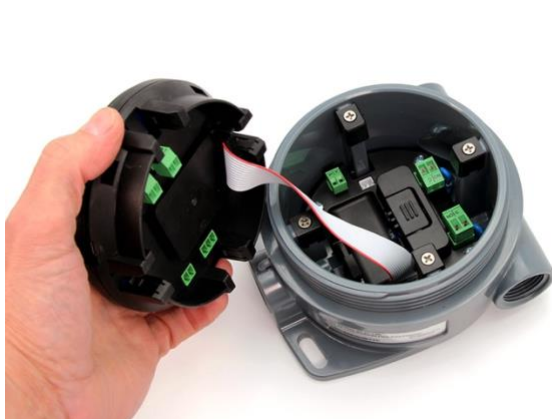
Options Module Mounted on the Bottom of Enclosure
