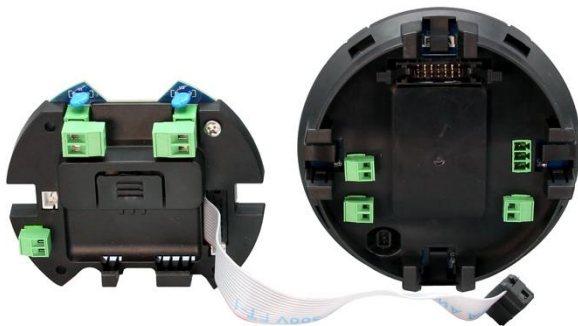
Options Board (Left) and Display Module (Right)
