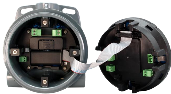
Options Board Connected to Display Module
