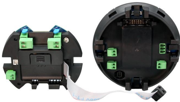
Options Board (Left) and Display Module (Right)
