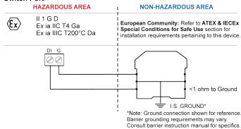
Switch Port Connection Entity Parameters: Ui = 30 V, Ii = 175 mA, Pi = 1 W, Ci = 0, Li = 0
