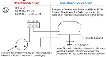
Loop/Power Connection Entity Parameters: Ui = 30 V, Ii = 175 mA, Pi = 1 W, Ci = 0, Li = 0
