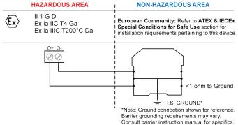
Open Collector Output Connection Entity Parameters: Ui = 30 V, Ii = 175 mA, Pi = 1 W, Ci = 0, Li = 0
