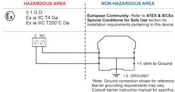
Relay Output Connection Entity Parameters: Ui = 30 V, Ii = 1.0 A, Pi = 1 W, Ci = 0.013  $\mu$ F, Li = 0 Uo = 11.55 V, Io = 0.001, A Po = 0.012 W
