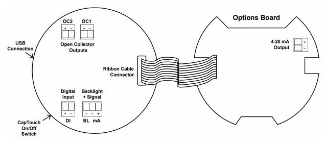
Figure 6. Connector Labeling for PD6907-HA-##-L3N
