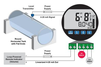
PD6907 Displaying Height in Feet and Volume in Gallons in a Round Horizontal Tank Using the Round Horizontal Tank Linearization Feature.
