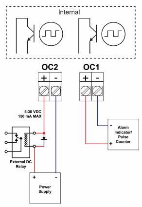
Figure 13. Open Collector Output Connections
