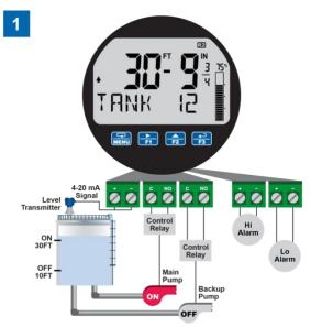
Relay #2 turns the main pump on at 30 feet and turns it off at 10 feet. 2 lights up to show relay 2 is energized. The findicates level is rising.
