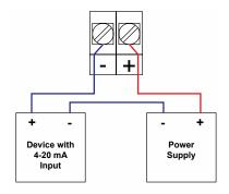
Figure 11. 4-20 mA Output Connections
