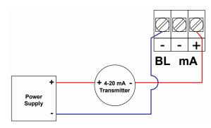
Figure 9. 4-20 mA Input Connection with Backlight
