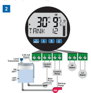
With the Pump Alternation feature activated, the next time the level reaches 30 feet, relay #1 transfers and starts the backup pump. 👪 lights up to show relay 1 is energized.
