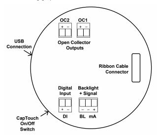
Figure 4. Connector Labeling for PD6907-HA-##-LNN
