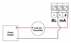
Figure 8. 4-20 mA Input Connection without Backlight
