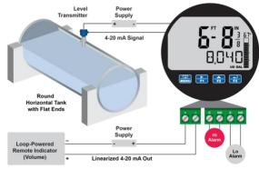
This function automatically calculates the volume in a round horizontal tank with flat ends and allows that reading to be displayed on the bottom display. This results in a meter that displays the height of the tank in convenient to read feet and inches on the top display and volume on the lower display. The user only needs to enter the diameter and length of the tank and the meter takes care of the rest.
