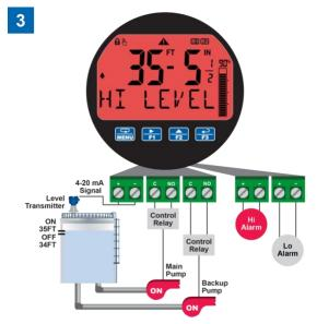
If the backup pump is not able to keep up, and the level reaches 35 feet, relay #2 transfers and starts the main pump as well. Open collector #1 trips the High Level Alarm, the display turns red and flashes "Hi Level" message, and indicates an alarm condition. The High Level Alarm resets at 34 feet.
