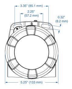
Figure 1. Enclosure Dimensions - Front View
