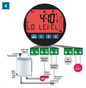
Once the level has dropped below the reset points, both relays will turn off. If the Main Pump fails to turn off, open collector #2 trips the Low Level Alarm at 5 feet to warn against the pump running dry. The Low Level Alarm resets at 6 feet.
