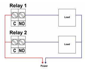
Figure 12. Solid-State Relay Connections
