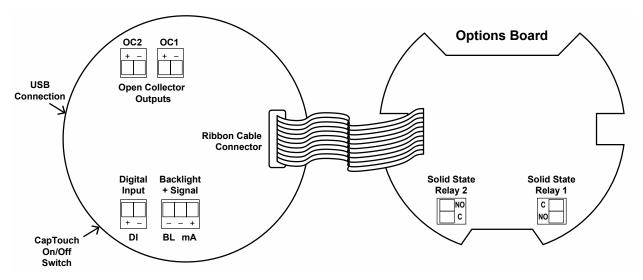
Figure 5. Connector Labeling for PD6907-HA-##-L2N
