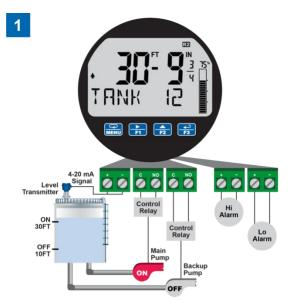
Relay #2 turns the main pump on at 30 feet and turns it off at 10 feet. 2 lights up to show relay 2 is energized. The • indicates level is rising.
