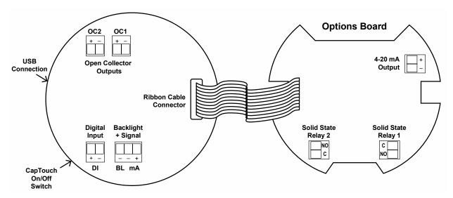
Figure 7. Connector Labeling for PD6907-HA-##-L5N
