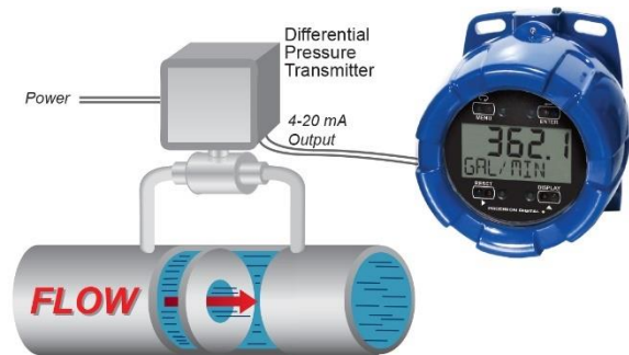
PD6820 Displaying Flow Rate by Extracting Square Root from DP Transmitter Signal.
