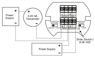
Figure 6. Connections with Externally-Powered Backlight
