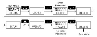
If the correct six-digit password is entered, the meter displays the message LINLDEKI (unlocked) and the protection is disabled until a new password is programmed.
