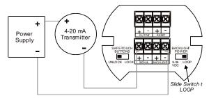
Figure 5. Connections with Loop-Powered Backlight
