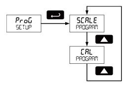
Note: The Scale and Calibrate functions are exclusive of each other. The meter uses the last function programmed. Only one of these methods can be employed at a time. The Scale and Calibrate functions can use up to 32 points (default is 2). The number of points should be set in the Advanced Features menu under the Multi-Point Linearization (LnERr) menu selection prior to scaling and calibration of the meter, see Advanced Features Menu, page 18.
