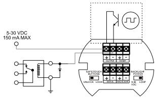
Figure 9. Output Connections
