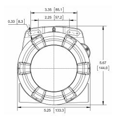
Figure 1. Enclosure Dimensions - Front View
