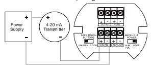
Figure 4. Connections without Backlight
