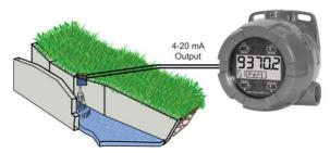
The PD6720, in combination with an ultrasonic level transmitter, makes for an economical way to measure and display open channel flow rate and total in most weirs and flumes. A guide such as the ISCO Open Channel Flow Measurement Handbook can provide the user with all the information needed: the exponent used in the flow equation for the desired flow units and the flow rate for any given head height.
