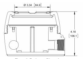
Figure 2. Enclosure Dimensions – Side Cross Section View
