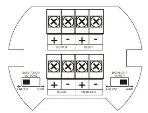
Figure 3. Connector Board
