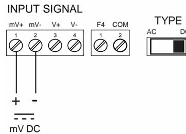
Figure 15. mV DC Connections
