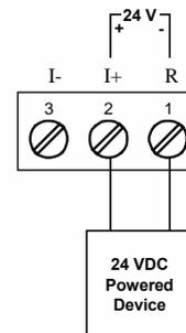
Figure 24. Analog Output Supply Powering Other Devices
