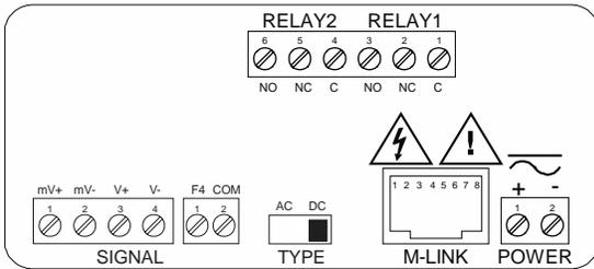
Figure 6. PD6402-##2 Connectors Label
