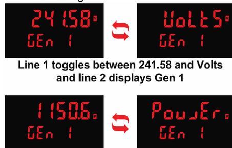
Line 1 toggles between 241.58 and Volts and line 2 displays Gen 1
