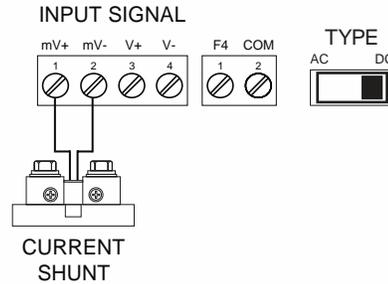
Figure 14. DC Current Shunt Connections
