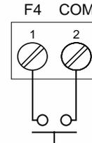
Figure 22. F4 Digital Input Connections
