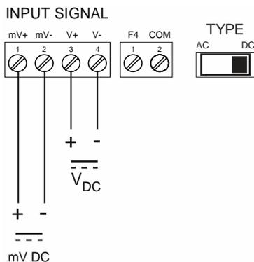
Figure 18. DC mV and High Voltage Connections
