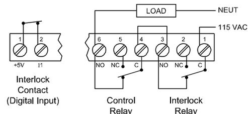
Figure 29. Interlock Connections
