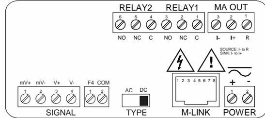
Figure 9. PD6402-##5 Connectors Label
