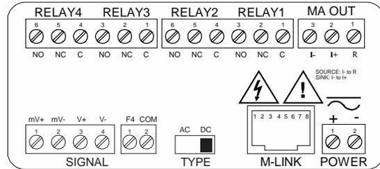
Figure 10. PD6402-##7 Connectors Label
