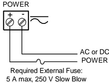
Figure 11. Power Connections
