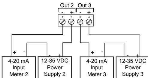
Figure 27. Dual 4-20 mA Output Module Connections
