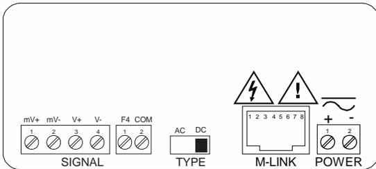
Figure 5. PD6402-##0 Connectors Label
