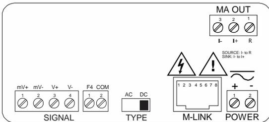
Figure 7. PD6402-##3 Connectors Label
