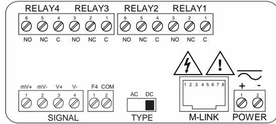
Figure 8. PD6402-##4 Connectors Label
