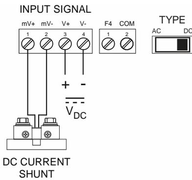
Figure 17. DC Current Shunt and Voltage Connections
