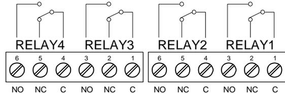
Figure 19. Relay Connections
