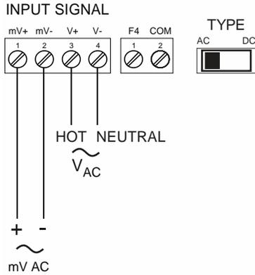
Figure 16. mV and High Voltage Connections
