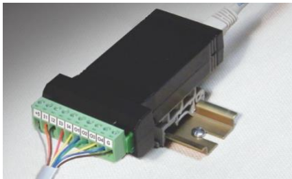
Figure 27. Expansion Module & DIN Rail Mounting Kit
