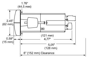
Figure 2. Controller Dimensions - Side View
