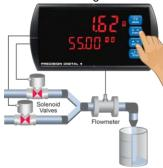
When the batch total reaches a value of 50.00 (Preset [55.00] – Pre-close [5.00]) the full-flow valve closes. The fill rate of the tank slows as a result.
