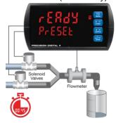
6. The new batch begins automatically after 60 seconds, both relays activate and both valves open.
