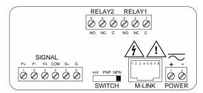
Figure 5. PD6310-##2 Connectors Label
