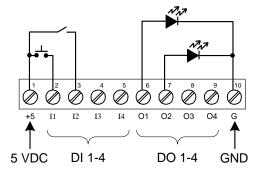
Figure 24. Digital I/O Module Connections
