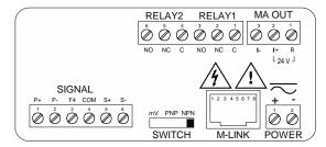
Figure 7. PD6310-##5 Connectors Label
