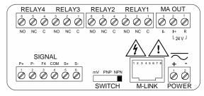
Figure 8. PD6310-##7 Connectors Label
