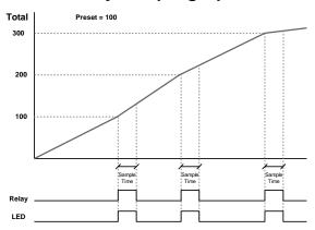
When the total reaches the preset, the relay trips and the sample time starts. After the sample time has elapsed, the relay resets. The cycle repeats every time the preset value is added to the total.
