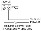
Figure 9. Power Connections
