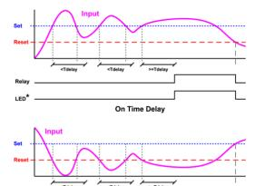
When the signal crosses the set point, the On time delay timer starts and the relay trips when the time delay has elapsed. If the signal drops below the set point (high alarm) before the time delay has elapsed, the On time delay timer resets and the relay does not change state. The same principle applies to the Off time delay.
