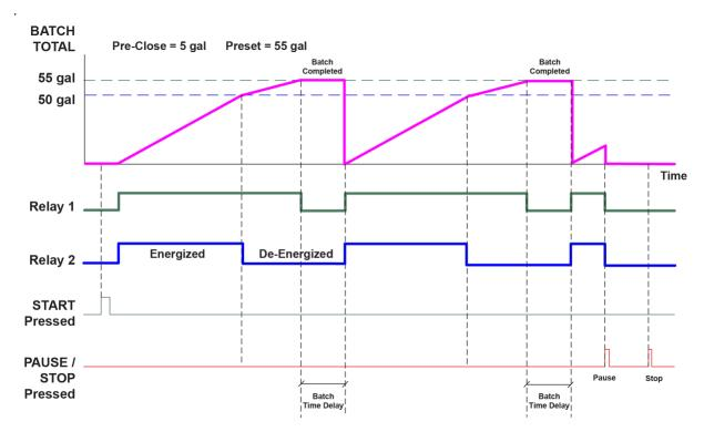
When START is pressed, a short delay occurs before the low flow alarm sensing is activated. Each relay can be programmed with additional ON delay to satisfy various conditions and applications.
