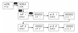
Note: The display values (d .5 1 and d .5 2) need to be in units of measure per second. For example, if the rate at 1000 Hz is 13.20 gal/min, this must be converted to gal/sec. In this scenario, the numbers input into the SCRLE menu would be as follows:
