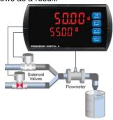
When the batch is complete, the restrictedflow valve closes. If overrun occurs, then the next batch will adjust for this offset amount to maintain accuracy.
