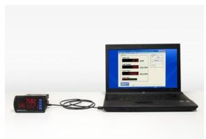
The controller can be powered from the USB connection. When using the USB connection, **DO NOT** apply AC or DC power to the controller.
