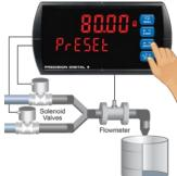
The new batch begins when the START button is pressed, so both relays activate and both valves open.
