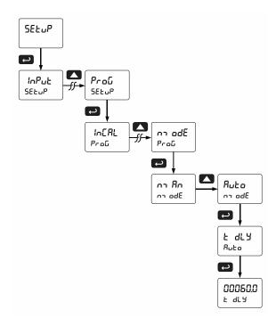
The time delay allows time for removing the full barrel and putting an empty barrel in place. Once the process starts, the operator does not have to press any buttons; except to pause or stop the batch process.
