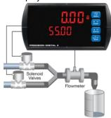
2. The START button is pressed. Both valves open. The barrel begins to fill.
