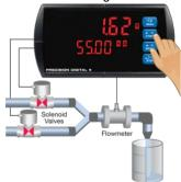
When the batch total reaches a value of 50.00 (Preset [55.00] – Pre-close [5.00]) the full-flow valve closes. The fill rate of the tank slows as a result.
