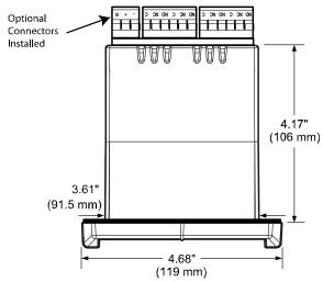
Figure 3. Controller Dimensions - Top View
