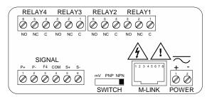
Figure 6. PD6310-##4 Connectors Label
