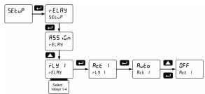
In the Advanced features – User menu program any of the digital inputs to Force On any of the internal relays (1-4).
