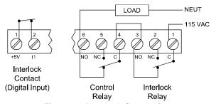
Figure 26. Interlock Connection
