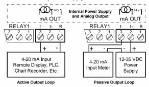
Figure 20. 4-20 mA Output Connections
