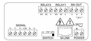
Figure 9. PD6300-##5 Connectors Label
