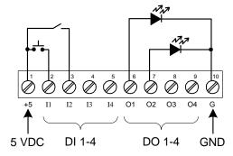
Figure 26. Digital I/O Module Connections
