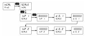
Note: The display values (d .5 1 and d .5 2) need to be in units of measure per second. For example, if the rate at 1000 Hz is 13.20 gal/min, this must be converted to gal/sec. In this scenario, the numbers input into the SERLE menu would be as follows:
