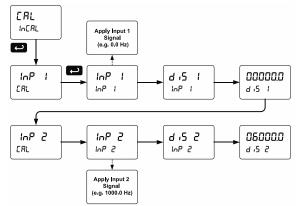
Note: The display values (d .5 / and d .5 Z) need to be in units of measure per second.
