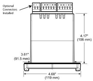
Figure 3: Meter Dimensions - Top View
