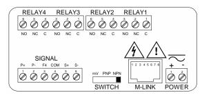
Figure 8. PD6300-##4 Connectors Label
