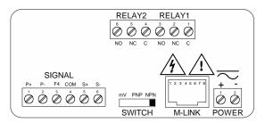
Figure 6. PD6300-##2 Connectors Label
