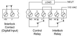
**Figure 28: Interlock Connections**
