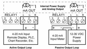
Figure 22: 4-20 mA Output Connections
