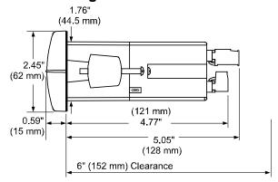
Figure 2: Meter Dimensions - Side View
