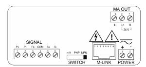
Figure 7. PD6300-##3 Connectors Label
