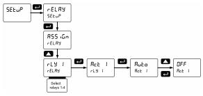
In the Advanced features – User menu program any of the digital inputs to Force On any of the internal relays (1-4).
