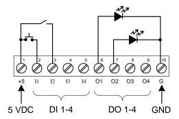
Figure 23. Digital I/O Module Connections
