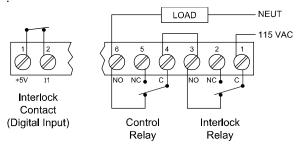
Figure 25. Interlock Connection
