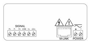
Figure 5. PD6200-##0 Connectors Label
