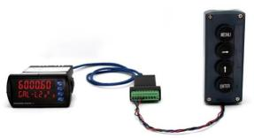
Figure 24. Meter to Control Station Connection
