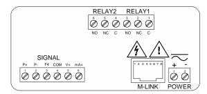
Figure 6. PD6200-##2 Connectors Label
