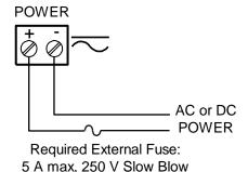
Figure 11. Power Connections
