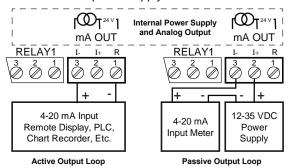
Figure 19. 4-20 mA Output Connections
