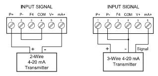
Figure 12. Transmitter Powered by Internal Supply
