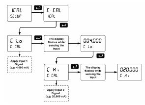
The graphic shows the calibration of the current input. The voltage input is calibrated in a similar way.
