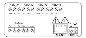
Figure 8. PD6200-##4 Connectors Label
