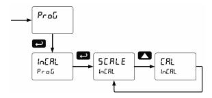
Note: The Scale and Calibrate functions are exclusive of each other. The meter uses the last function programmed. Only one of these methods can be employed at a time. The Scale and Calibrate functions can use up to 32 points (default is 2). The number of points should be set in the Advanced menu prior to scaling and calibration of the meter. See Multi-Point Linearization (Line Rr) on page 41 for details.
