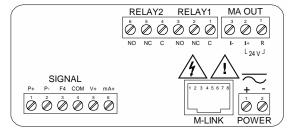
Figure 9. PD6200-##5 Connectors Label
