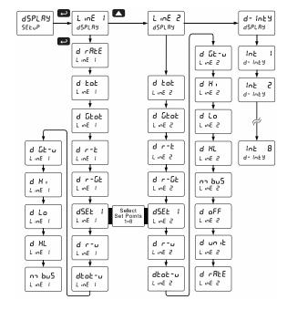
Selecting engineering units or custom legends as display line 2 (d unit) will display the unit or tag selected for the rate, total, or grand total displayed on line 1.
