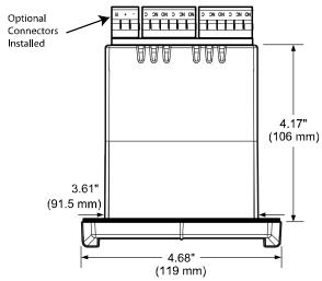
Figure 3. Meter Dimensions - Top View
