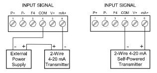
Figure 13. Transmitter Powered by External Supply or Self-Powered
