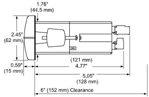
Figure 2. Meter Dimensions - Side View
