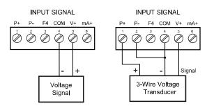
Figure 14. Voltage Input Connections
