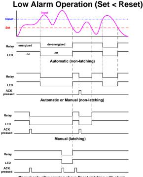
Manual only after passing above Reset (latching with clear) For Manual reset mode, ACK can be pressed anytime to turn "off" relay. For relay to turn back "on", signal must go above set point and then go below it.
