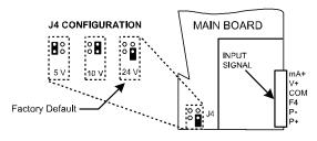
Figure 5. Transmitter Supply Voltage Selection
