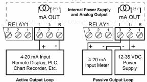
Figure 20. 4-20 mA Output Connections
