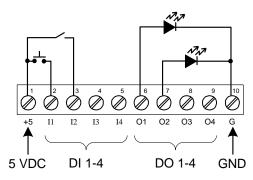
Figure 24. Digital I/O Module Connections
