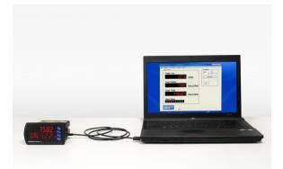
The meter can be powered from the USB connection. When using the USB connection, <u>**DO NOT**</u> apply AC or DC power to the meter.
