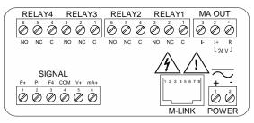
Figure 11. PD6000-##7 Connectors Label
