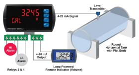
Set the display for the desired decimal point and engineering units before entering the round horizontal tank function. Select units, inches or cm for the tank dimensions. Enter the diameter and the length in inches and the results are calculated automatically in US gallons. Enter the diameter and length in cm and the results are calculated automatically in liters. The meter can be scaled to display the volume in any engineering unit.
