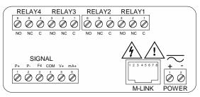
Figure 9. PD6000-##4 Connectors Label
