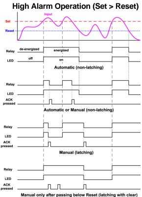
For Manual reset mode, ACK can be pressed anytime to turn "off" relay. To detect a new alarm condition, the signal must go below the set point, and then go above it.
