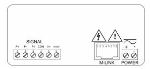
Figure 6. PD6000-##0 Connectors Label
