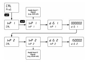
Note: Inputs for the above example are: Input 1: 4.00 mA; Display 1: 0.0 Gallons Input 2: 20.00 mA; Display 2: 15000.0 Gallons
