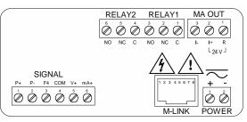
Figure 10. PD6000-##5 Connectors Label
