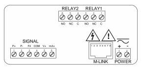
Figure 7. PD6000-##2 Connectors Label
