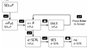
Set d-SLRL to no if only one scale is needed for the input.
