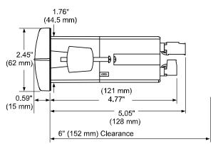
Figure 3. Meter Dimensions - Side View
