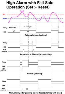
Manual only after passing below Reset (atching with clear) Note: Relay coil is energized in non-alarm condition. In case of power failure, relay will go to alarm state.
