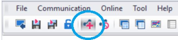
Select the communication port, protocol, baud rate, serial communications parameters, and addressed of the controller(s) connected. Once the configuration is complete, select Add Port.
