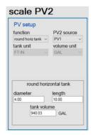
MeterView XL Round Horizontal Tank Function Automatically Calculates the Volume Once the Diameter and the Length of the Tank are Entered.
