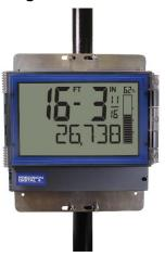
PD4-6603 Meter Shown mounted to pipe using PDA6260 pipe mounting kit. See *Pipe Mounting Instructions* on page *20* for details.
