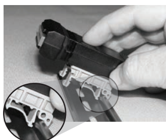
Figure 8. Snapping the Module to the DIN Rail
