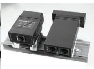
Figure 9. Typical Installation of DIN Rail Mounted Devices
