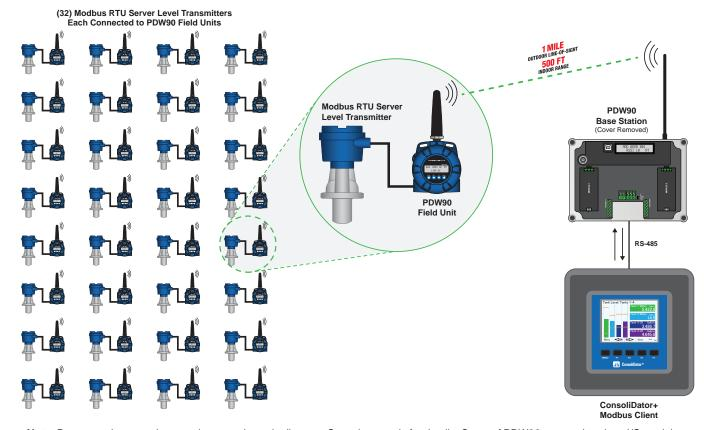
Note: Power requirements / connections not shown in diagram. Consult manuals for details. Cover of PDW90 removed to show I/O modules.
