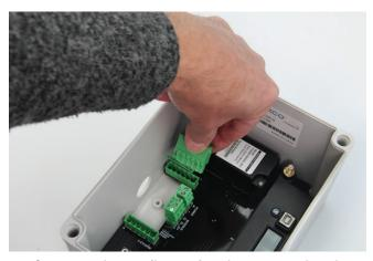
Connector plugs easily snap into the connector board.
