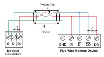
**Base Station Five-Wire RS-485 Modbus Connections**
