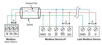
Base Station Multiple Device RS-485 Modbus Connections
