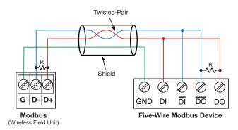
Field Unit Five-Wire RS-485 Modbus Connections
