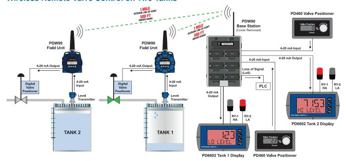
Note: Power requirements / connections not shown in diagram. Consult manuals for details. Cover of PDW90 removed to show I/O modules.
