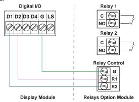
**Note:** Connections between relay control connection and relays are with traces on PCB.
