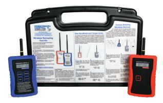
The handheld and target units are used to survey wireless signal strength throughout nonhazardous ar-eas of a facility prior to PDW30 or PDW90 equipment installation. The target unit is set in a desired installation location and the handheld is brought to another installation location. The handheld unit will provide an indication of signal strength between the two units.
