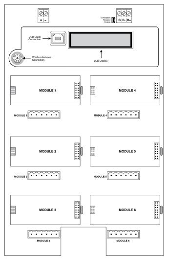
6-Module Base Station Sub Panel (Connector Board)
