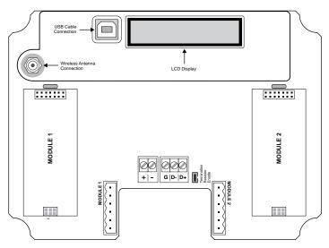
2-Module Base Station Sub Panel (Connector Board)
