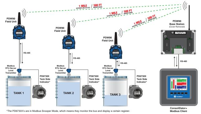
Note: Power requirements / connections not shown in diagram. Consult manuals for details. Cover of PDW90 removed to show I/O modules.
