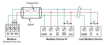
Field Unit Multiple Device RS-485 Modbus Connections
