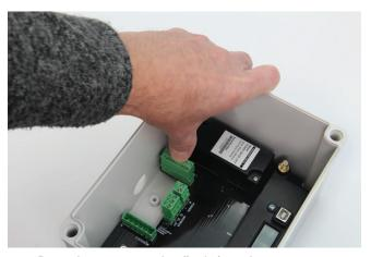
Press the connector plug firmly into place to secure.
