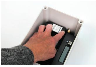
Press the module firmly into place to secure.
