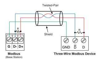
Base Station Three-Wire RS-485 Modbus Connections
