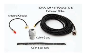
The PDWA3120-N and PDWA3140-N are 20-foot and 40-foot extension cables used to extend the distance between the Yagi Antenna and the PDW30 or PDW90 wireless units. The extension cables also come with an antenna coupler to connect the PDW wireless device to the antenna extension cable, coax seal tape, and a 3/4" NPT cable gland.
