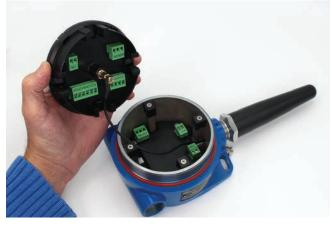
Relays Option Module Mounted on the Bottom of Enclosure (Install the module using the four screws provided)
