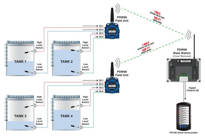
Note: Power requirements / connections not shown in diagram. Consult manuals for details. Cover of PDW90 removed to show I/O modules.
