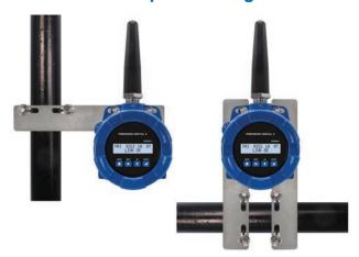
The PDWA6963-SS provides a convenient way to mount one PDW30 primary/secondary, PDWR repeater, or PDW90 field unit to a horizontal or vertical 1.5" or 2" pipe such that the antenna is not right on top of the metal pipe.
