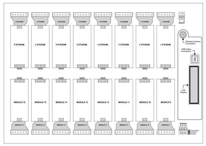
16-Module Base Station Sub Panel (Connector Board)
