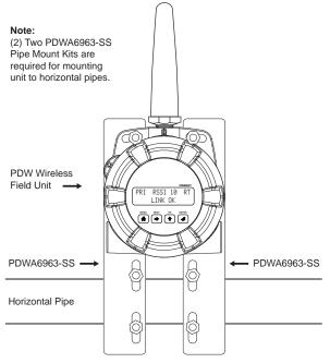
PDW Unit Mounted to Horizontal Pipe with Two PDWA6963-SS Kits
