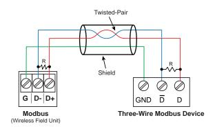
Field Unit Three-Wire RS-485 Modbus Connections
