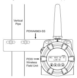
PDW Unit Mounted to Vertical Pipe with One PDWA6963-SS Kit
