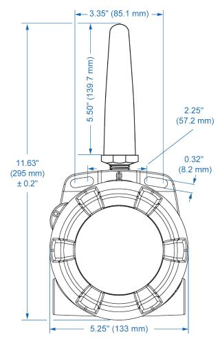
**Enclosure & Antenna Dimensions - Front View**
