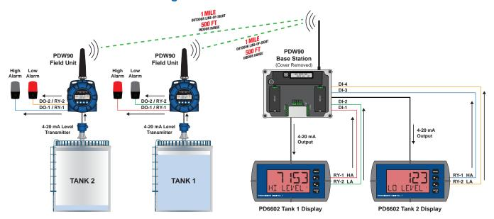
Note: Power requirements / connections not shown in diagram. Consult manuals for details. Cover of PDW90 removed to show I/O modules.
