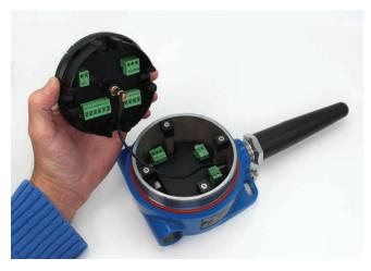
Relays Option Module Mounted on the Bottom of Enclosure (Install the module using the four screws provided)
