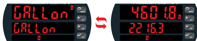
Lower Display Alternating Input Channels A & B Totals
