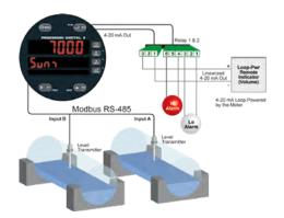
**Round Horizontal Tank Signal Input Conditioning**
