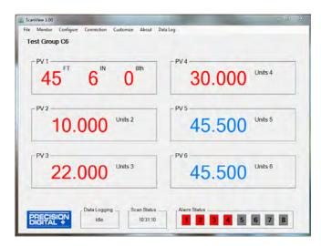
Once the scanner has been configured, the user chooses Monitor from the top menu bar. The Monitor window will appear; the enabled PVs and all associated values will take a few seconds to display.
