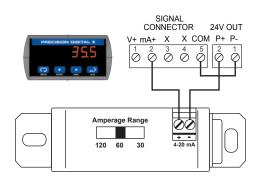
PDA6420 powered by PD603-6R0-1. The PD603 displays the current measured by the PDA6420.
