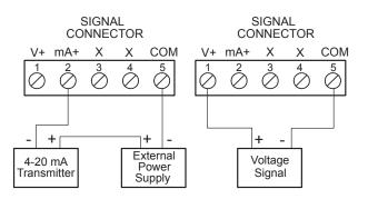
**Transmitter Powered by External Supply**
