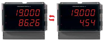
Lower Display Alternating Input Channels A & B
