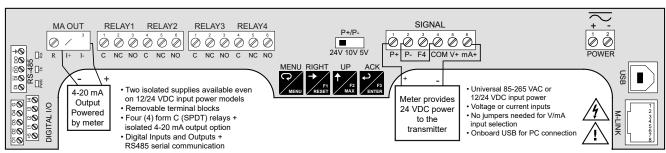
Connector Labeling for Fully Loaded PD2-6000
