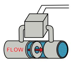
In this application, the PD2-6000 is displaying flow rate by extracting the square root from the 4-20 mA signal from a differential pressure transmitter. The user selectable low-flow cutoff feature gives a reading of zero when the flow rate drops below a user selectable value.
