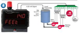
Relay #3 trips the High-Level Alarm at 14.0 feet and resets at 10.0 feet. The optional light starts flashing and the horn sounds.
