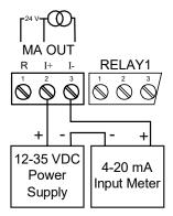
4-20 mA Output Powered by External Power Supply
