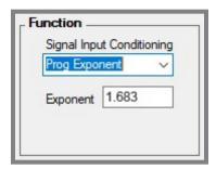
The input is raised to an exponent progrmmable by the user resulting in a display of open channel flow rate.
