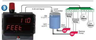
If the backup pump is not able to keep up, and the level reaches 11.0 feet, relay #1 transfers and starts the main pump as well.
