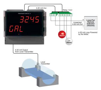
In this application, a level sensor is measuring the height in the round horizontal tank and the Helios is converting that signal to volume using the RHT function. All the user has to do is input the diameter and length of the tank and the meter converts the signal to volume.
