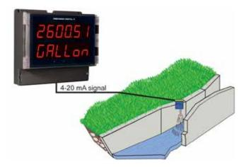
In this application, a level sensor is measuring the height in a weir and the Helios is converting that signal to flow rate using the programmable exponent function. All the user has to do is input the corresponding exponent for their weir and the meter will convert the signal to flow.
