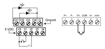
4 Digital Inputs F4 Terminal for & 4 Digital Outputs **Digital Input**
