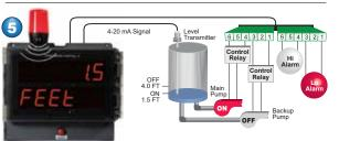
Relay #4 trips the Low-Level Alarm at 1.5 feet and resets at 4.0 feet. The optional light starts flashing and the horn sounds.
