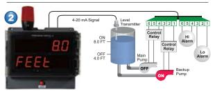
With the Pump Alternation feature activated, the next time the level reaches 8.0 feet, relay #2 transfers and starts the backup pump.
